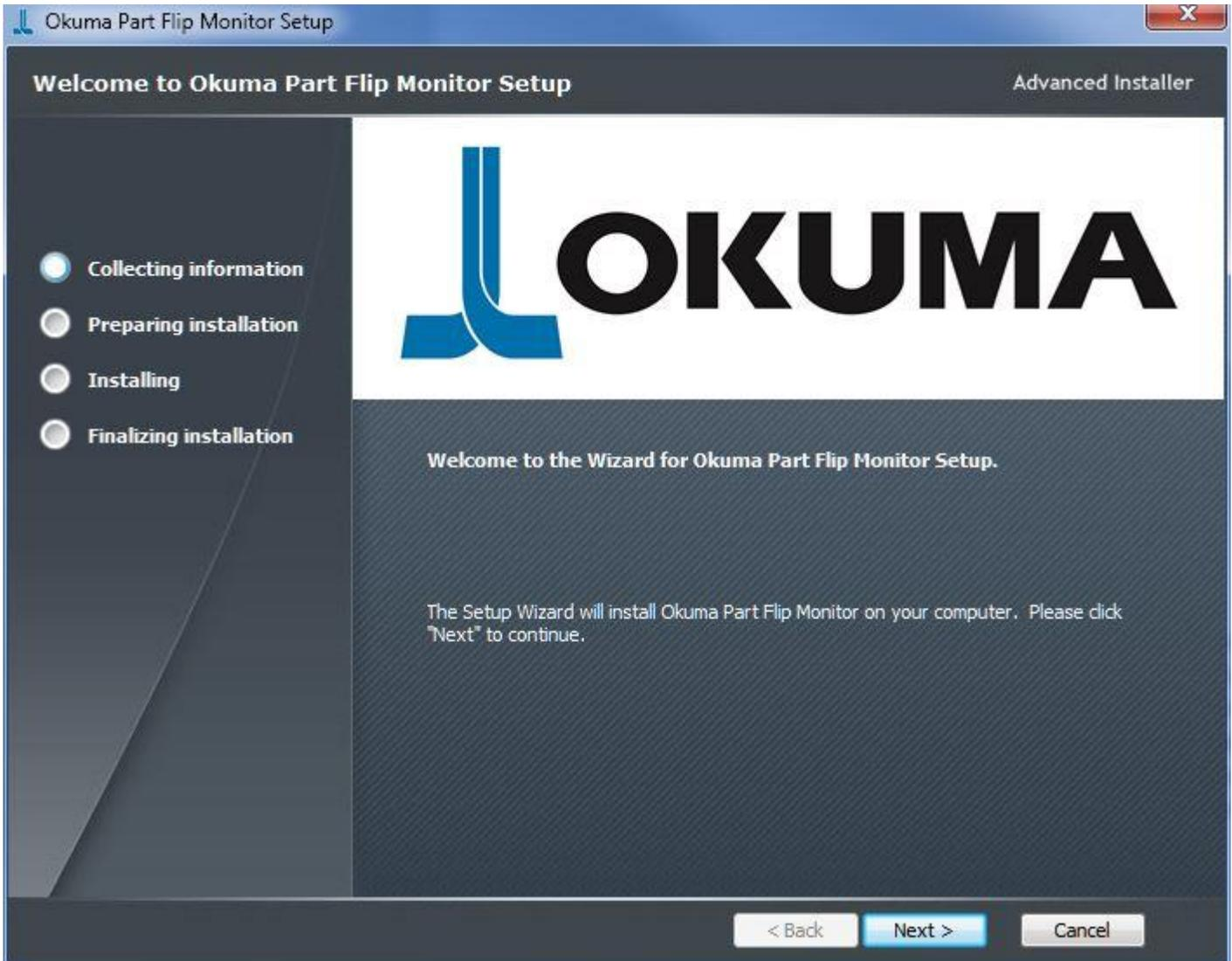
After downloading the application from the Okuma App Store, run 'Setup\_OkumaPartFlipMonitor.exe, click 'Next >' to go through the installation wizard and have the application installed. For subsequent application starts, simply open to the start menu and look for the 'Okuma Part Flip Monitor' program group. The uninstall application can be found in both the control panel (Add/Remove application) and the start menu under 'Okuma Part Flip Monitor'.
