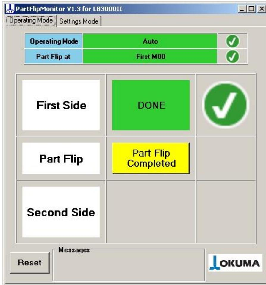
When the “Require user confirmation after part flip” is checked in the Setting Mode tab, as soon as the first side is completed the application will disable the Cycle Start and the “Part Flip Completed” button will appear next to “Part Flip”. Once the part is flipped, press this button in order to flag the part flip as done and the application will enable the Cycle Start for executing the Second Side. This is the only mode available when the application is used on machining centers.
