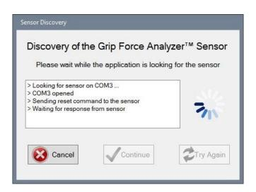
The Sensor Discovery scans trough every Serial Communication port trying to find the sensor. On a system with 2 serial ports, it normally takes about 30 seconds. If there are more serial ports, the time will increase accordingly. While the loading animation is running, the Sensor Discovery is working and giving feedback messages.
