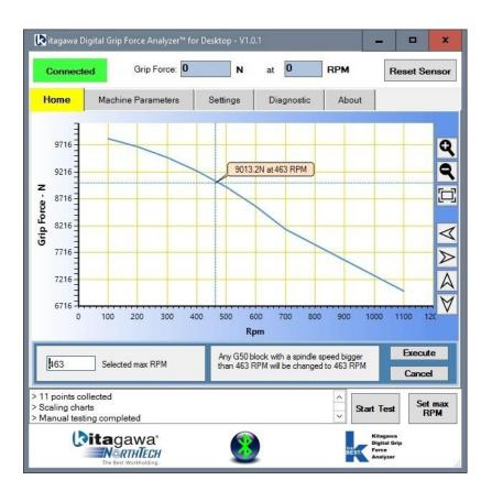
Whit this functionality the application can automatically set the maximum RPM in the user part program, accordingly with the maximum loss of grip force allowed by the user.
