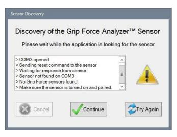
Sometimes, the sensor discovery cannot find the sensor. Make sure the USB dongle is properly plugged in and that the sensor is ON. Press the *Try Again* button to run the Sensor Discovery one more time. If still the Sensor Discovery cannot find the sensor, follow this procedure:
