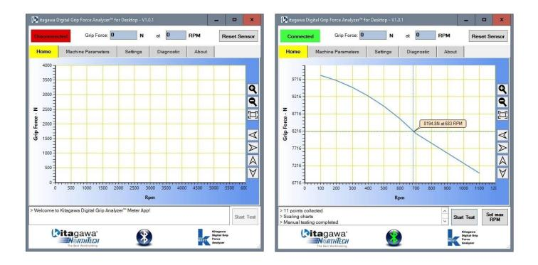
When the application is started for the first time, the chart is empty and the connection with the sensor is not active. The 5 tabs: *Home, Machine Parameters, Settings, Diagnostic* and *About,* are explained in details in the next paragraph. The Automatic Test and Manual Test buttons are enabled only when the application is connected to the sensor.
