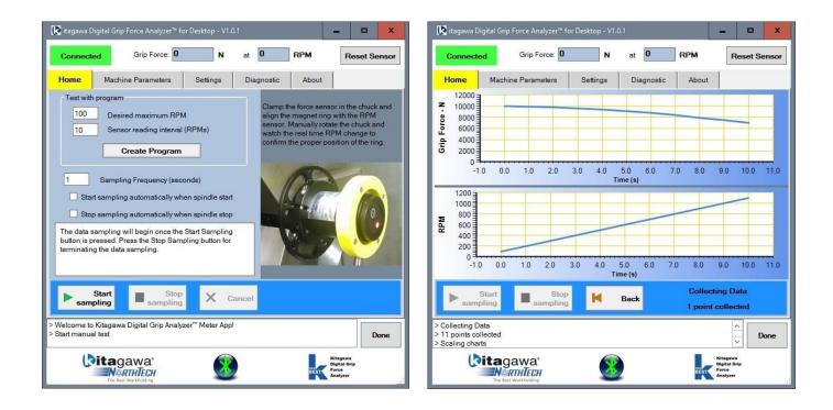
The Manual Test is used to record data on the fly by spinning the spindle manually, either in manual mode with the spindle override or in MDI mode by programming the desired spindle RPM. In the Manual Test mode, the setting needed are the sampling frequency in seconds, and if the application will start and/or stop the sampling automatically. The default sampling frequency is 1 second, meaning that the application will read the grip force and RPM once per second.
