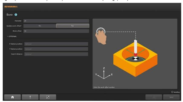
The app generates the required G-code program and loads it to the NC, either as the main program or in MDI mode (dependent on the *Upload type* selected during configuration).
