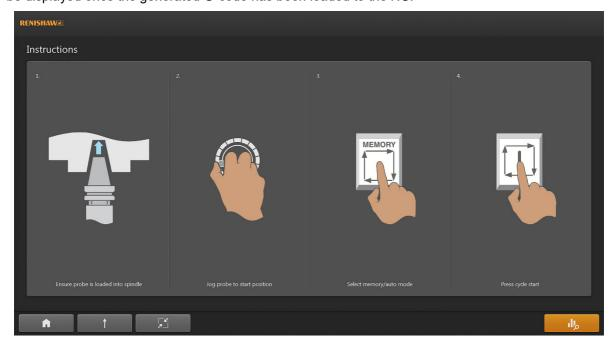
Follow the on-screen instructions to put the machine into the correct mode and press cycle start.
