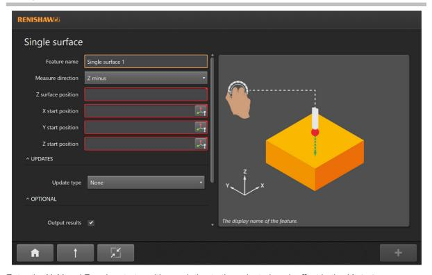
Enter the X, Y and Z probe start positions relative to the selected work offset in the *X start position*, Y start position and Z start position fields.
