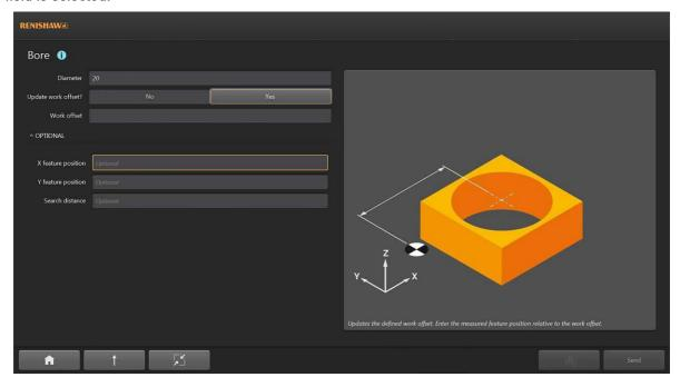
Once all required values have been entered into the cycle, load the probe to the machine spindle (if not already loaded).
