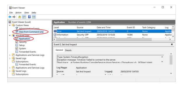
Set and Inspect errors or warnings can be identified by looking for 'Set and Inspect' in the *Source* column.
