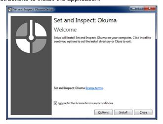
The set-up process will install all required system components – such as the .NET 4.0 framework and the Set and Inspect application – to the target CNC machine tool control, and create a desktop shortcut.
